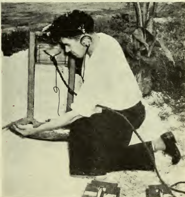
Charles Hedden with an early model of the treasure locator which evolved into the magnetic mine detector shown above
